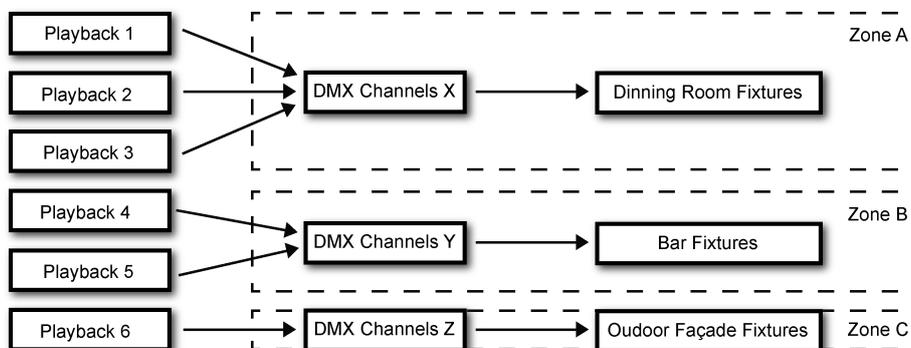
Figure 9.3: Playbacks controlling zones in a restaurant
