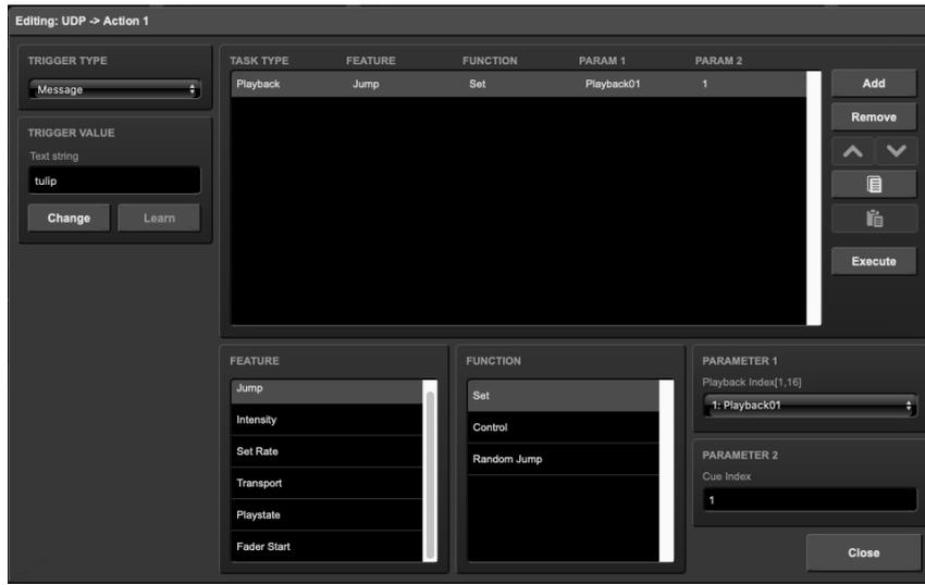
Press the 'Close' button, select the second action and press 'Edit' again. Change this trigger value to "crocus". Add a task by pressing 'Add' and choose the 'Playback' task-type. Select the newly added task and set the 'feature' to 'Transport' and set the 'function' to 'Jump'. Parameter 1 should be set to '1' (addressing the first playback) and parameter 2 should be set to '2' (jump to the second cue).
