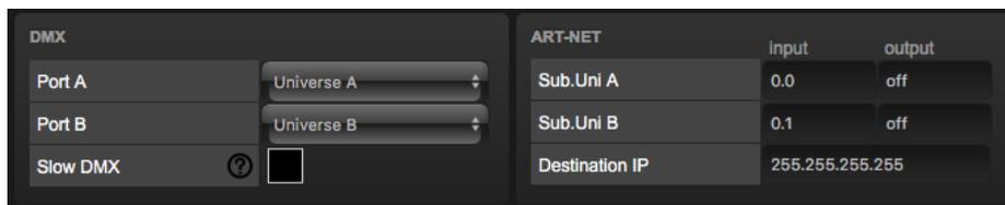
Figure 11.6: Converting Art-Net to DMX step 3
