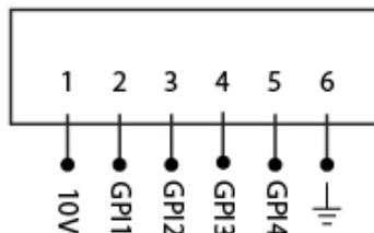
Figure 4.4: GPI Pinout
