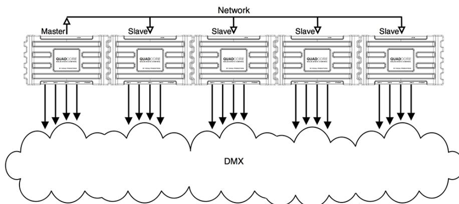
Figure 6.3: Master/Slave setup
