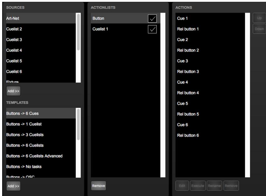
Pressing the buttons 1 till 3 will now activate cues 1 till 3. The button's LEDs will indicate which cue is active.
