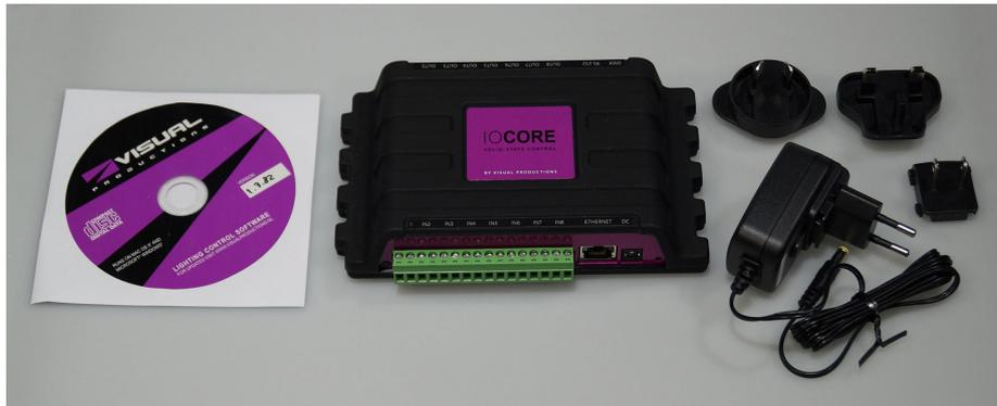
Figure 1.2: IoCore1 box contents
