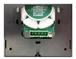
Figure 2.3: Terminal connector, seen through the backplate
